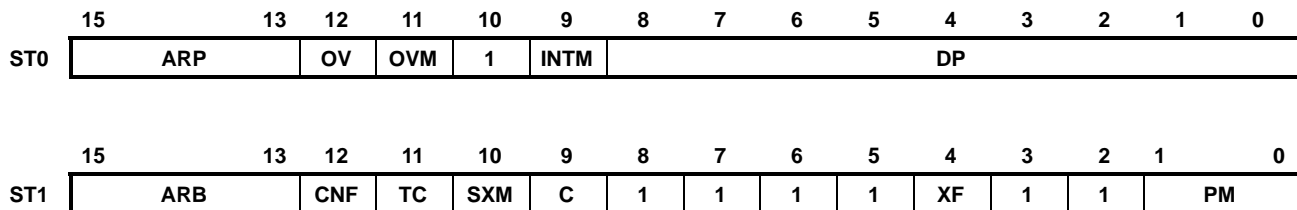
Figure 10. Status and Control Register Organization
